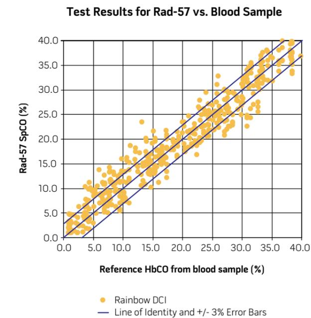
Masimo Rainbow SET is clinically proven to measure COHb saturation in the range of 0 to 40% with accuracy of +/-3% (1 S.D.). This encompasses 67% of the data.
