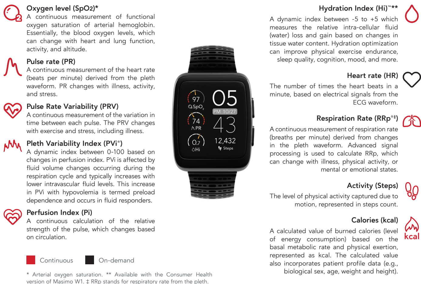
Figure 2. Physiological Parameters Measured Continuously (Red) and On-demand (Blue) by Masimo W1
